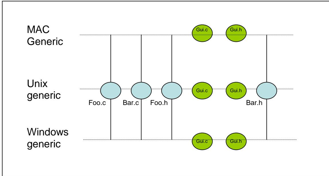
In this case, the files Gui.c and Gui.h are different for each operating system and must remain diverged. The MAC, Unix and Windows generics all share the vast majority of files and only the files necessarily different to implement the GUI on each OS are diverged.
