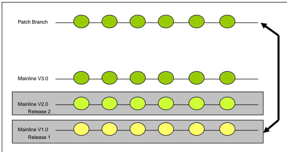
In this example, release 1.0 has been extracted into a new generic called the patch branch. The generic is locked and all of the files that are edited to resolve the problem are either already uncommoned or will become uncommoned as part of the edit operation.
