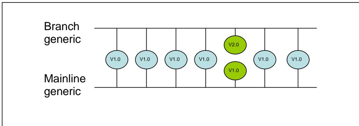
In this example, the green circles represent a single uncommoned file. Each branch contains a separate physical instance of this file and shared instances of all the other files. When the files are **recommoned**, a single file instance will again be shared by both branches.
